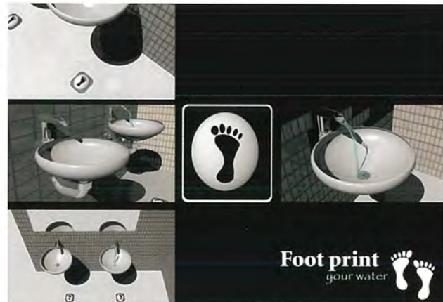
'Foot print your water' was designed to reduce the water lost in a bathroom sink, as the sustainable foot pedal would allow a constant flow
