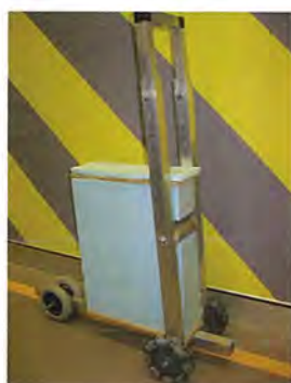
Mock-up model made from aluminium extrusions
