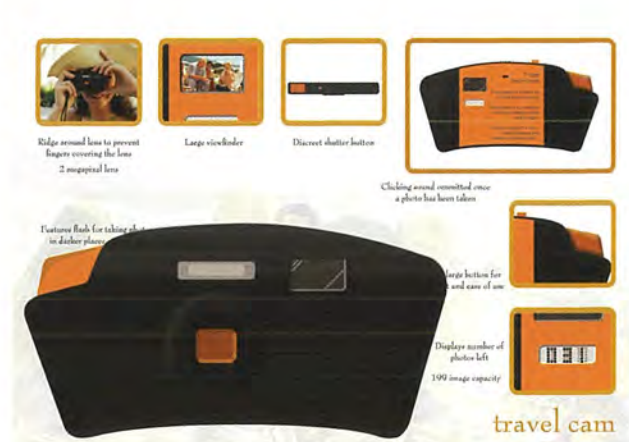
Digital Camera - This is a variation of the same project featuring a flash which also doubles as a torch for improved night time photos
