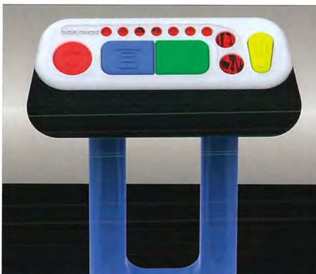
User interface. Three step interaction for forward motion: Turn on bipod (left red button), Select movement type (intermittent - blue or continuous - green) dependent on user's physical condition, and handle buttons for ignition. LED array displaying battery life and light button (yellow) for night use
