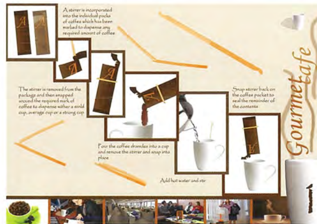
Cormack Packaging - Designed for Cormack Packaging Awards aimed at improving existing packaging. This instant coffee sachet is re-sealable and includes a stirrer
