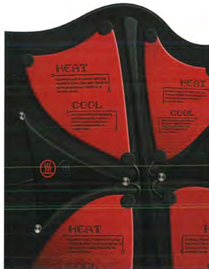
The removable heat and cooling packs and circuitry packs are clipped into the garment, with each describing its function graphically
